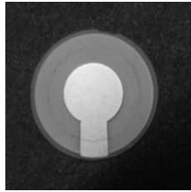
Fig. 1 GaPO 4 thickness shear resonator with gold electrodes (10 mm diameter)
